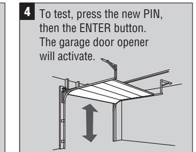
**4** To test, press the new PIN, then the ENTER button. The garage door opener will activate.
