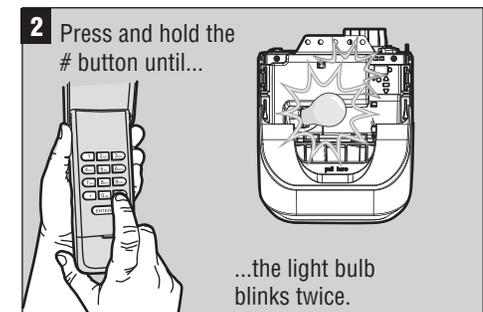
**2** Press and hold the # button until... ..the light bulb blinks twice.
