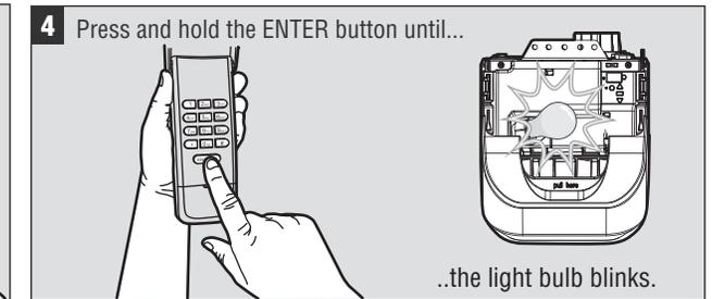
**4** Press and hold the ENTER button until... ..the light bulb blinks.
