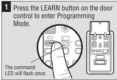
**1** Press the LEARN button on the door control to enter Programming Mode. The command LED will flash once.
